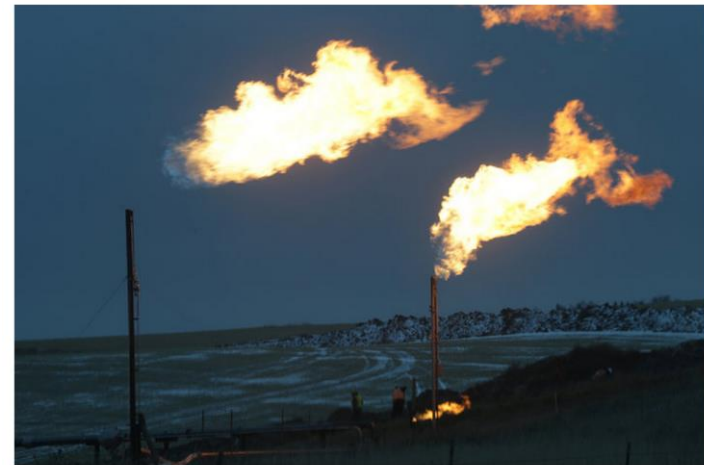
Flares burning waste gas at a well in McKenzie County, N.D., in the Bakken shale oil field. Jim Wilson/The New York Times
